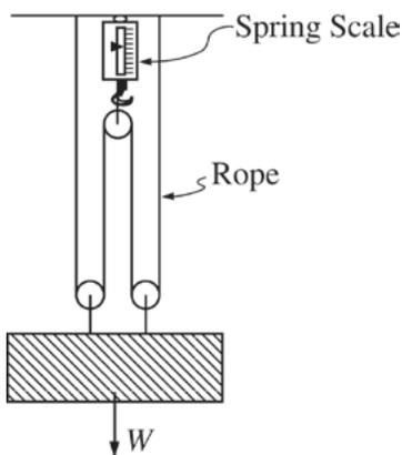
24. The rope-and-pulley system of negligible mass shown above supports a block of weight  $W$  that is at rest. If the tension throughout the rope is uniform, what is the reading on the spring scale?
