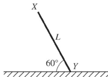
25. The uniform rod of length  $L$  shown above is supported by holding end  $X$  so that the rod makes an angle  $60^\circ$  with the horizontal floor. There is no friction acting between the rod and the floor. When the support at  $X$  is removed, the rod falls under the influence of gravity. Which of the following best describes the movement of end  $Y$  as the rod falls?
