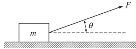
23. A block of mass  $m$  is pulled across a rough horizontal surface at constant speed by a force of magnitude  $F$ , which acts at an angle of  $\theta$  to the horizontal, as shown above. The coefficient of kinetic friction between the block and the surface is
