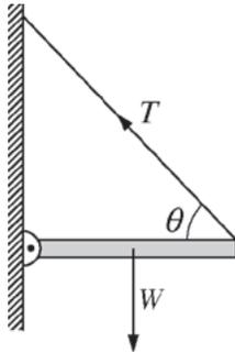
18. A uniform beam of weight  $W$  is attached to a wall by a pivot at one end and is held horizontal by a cable attached to the other end of the beam and to the wall, as shown above.  $T$  is the tension in the cable, which makes an angle  $\theta$  with the beam. Which of the following is equal to  $T$ ?
