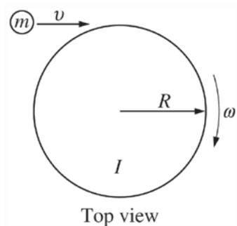
35. A circular platform has a radius  $R$  and rotational inertia  $I$ . The platform rotates around a fixed pivot at its center with negligible friction and an initial angular velocity  $\omega$ . A child of mass  $m$  (represented by the small circle in the figure above) runs tangentially with speed  $v$  and jumps on the outer edge of the platform. When the child is standing on the outer edge of the platform, the new angular velocity is
